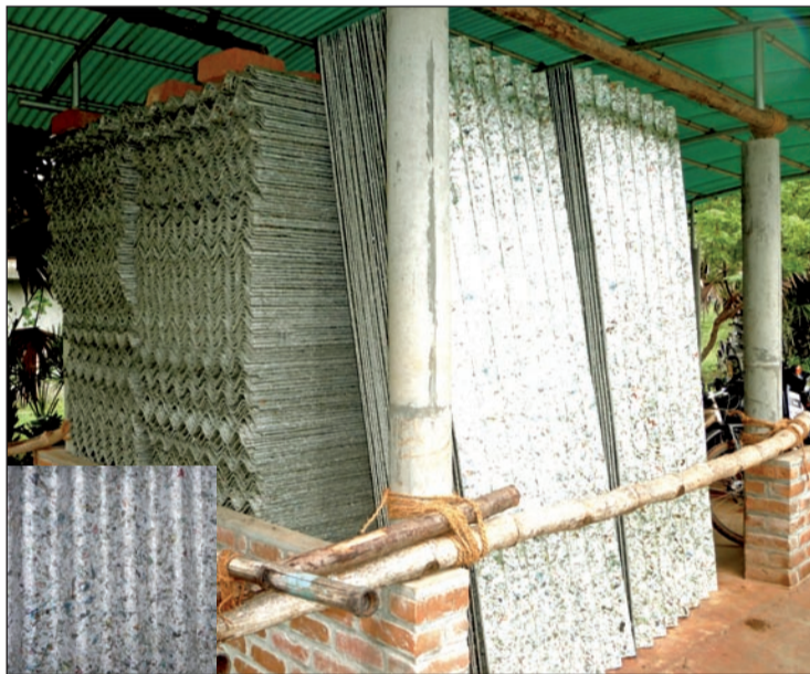
Corrugated roof panels made from recycled TetraPaks
